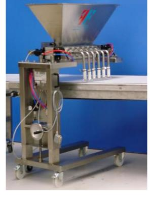
The Form & Frys piston filling machine is built as a roll in roll out unit on a height adjustable "C" frame allowing it to be used in various positions.
